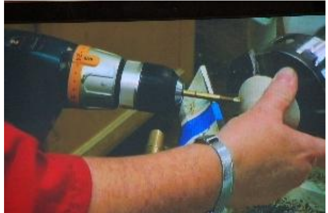
Drilling the 3 equally spaced and angled holes for the whistles (not pictured)
