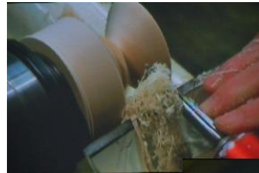
Shaping the outside of the body of the top
