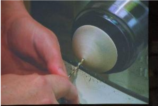
Drilling the hole for the hardwood tip
