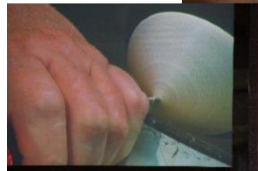
Preparing to drill a hole for the tip (different hardwood)
