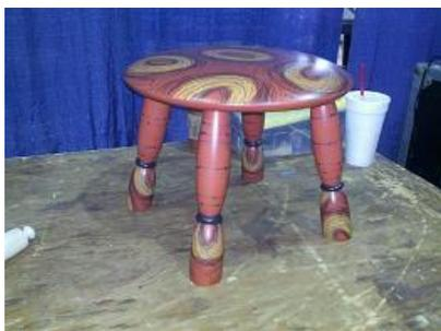
jig to hold the seat at the correct angle. When shaping the leg tenons, she said a mechanics open end wrench made a good caliper. Regarding glue, if the joint was tight she used yellow glue. If the fit was sloppy, she used epoxy. Nick Cook manned the camera during the demonstration. Kimberly mentioned that Nick has a very good article on his web site on turning a stool for anyone in the audience wanting more information.
