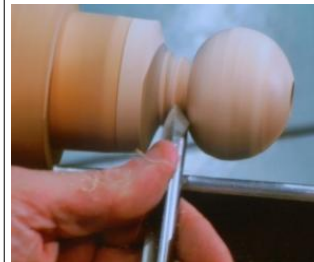
Using a 3/8" detail gouge to finish the shaping and to separate the body from the waste. Sand with 120, 180, 240, 320, 400. Higher if using exotic wood.
