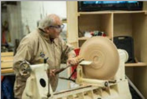
After shaping the bottom of the platter he created a recess to reverse chuck the platter and to finish the front side.
