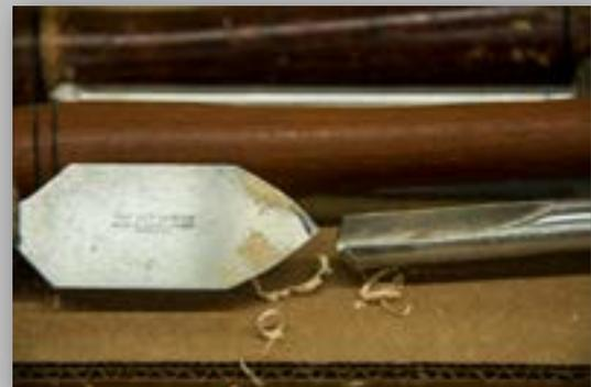
Two of the tools that Ray used in making the platter: A diamond shape scraper and a blunt end gouge.
