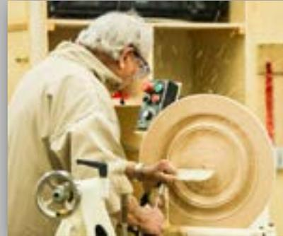
Ray said that his rule of thumb was that the width of the rim (total of both sides of the platter) should equal approximately 1/4 the width of the platter. So, for this platter, which was 19 1/2 inches wide, the rim on each side should be slightly less than 2 1/2 inches.
